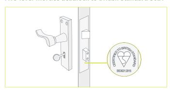
A five-lever mortice deadlock is a key-operated door lock commonly found on timber doors. **You** can easily identify if **Your** mortice deadlocks are to British Standard as they will have the British Standard Kitemark engraved on the faceplate of the door with 'BS3621' underneath. British Standard 3621 deadlocks must be five-lever, so if **Your** lock features the Kitemark it will meet **Our** minimum security requirements.
