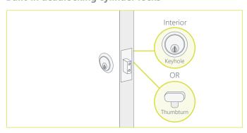
These locks are commonly found on PVCu doors. They have a square-ended deadbolt and can lock from one or both sides by key. Some cylinder deadlocks only lock by key from the outside, whilst inside the lock is operated by a thumbturn. **You** may have a single-entry deadlock which is only operable from the outside and has no keyhole on the interior side. All locking styles are acceptable to meet **Our** minimum security requirements.
